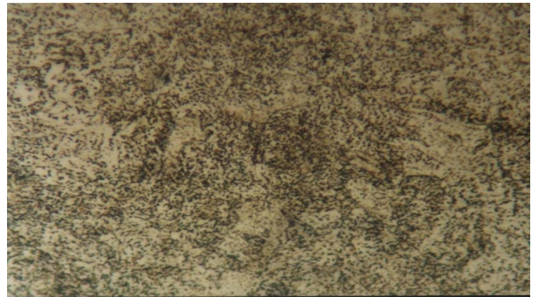
AISI 4340 Low alloy steel, Brightfield Magnification: 800X Etching: 4% Nital
